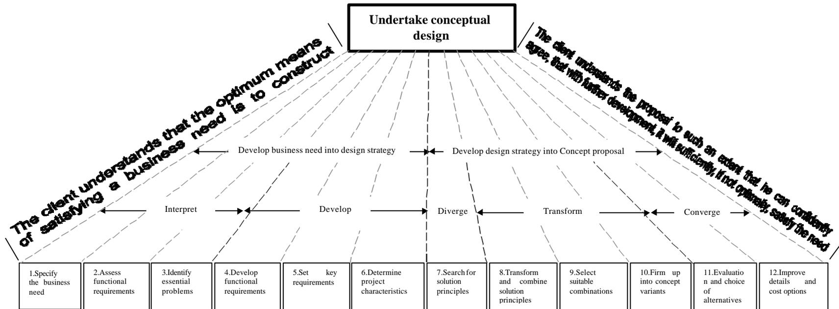
**Figure 1**      The preliminary conceptual design framework model
