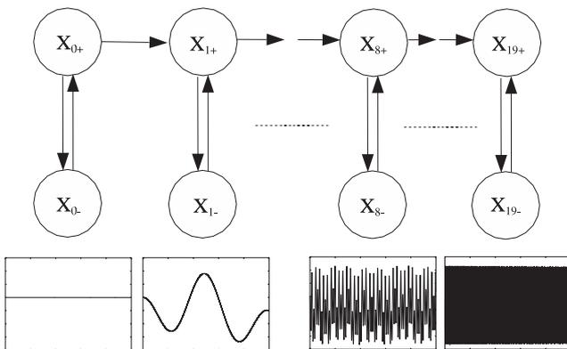
**Fig. 4.** The cascade oscillators demonstration model. The model has a basic unit of two variables coupled by the following equations:  $d[X_{i+}]/dt = -k2^i[X_{i-}] + k2^{i-1}[X_{(i-1)-}]$ ,  $d[X_{i-}]/dt = k2^i[X_{i+}]$  where  $k$  is a time scaling factor. A cascade has 20 instances of the unit. The model has five sets of the cascade. Four sample solutions of the cascade oscillators model are shown below the first (slowest), second, ninth and twentieth (fastest) components.
