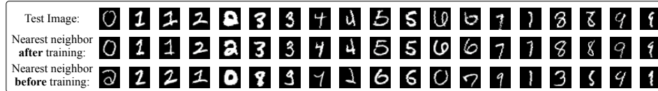
Figure 4: Top row: Examples of MNIST images whose nearest neighbor changes during training. Middle row: nearest neighbor after training, using the Mahalanobis distance metric. Bottom row: nearest neighbor before training, using the Euclidean distance metric.
