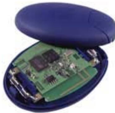
**Figure 4: Bluetag.** Bluetooth based smart-tag.
