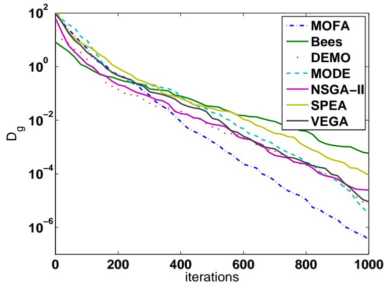
Figure 9: Convergence comparison for the disc brake design.
