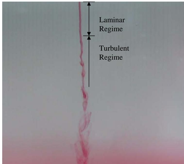
Figure 3 Typical picture of the flow development
