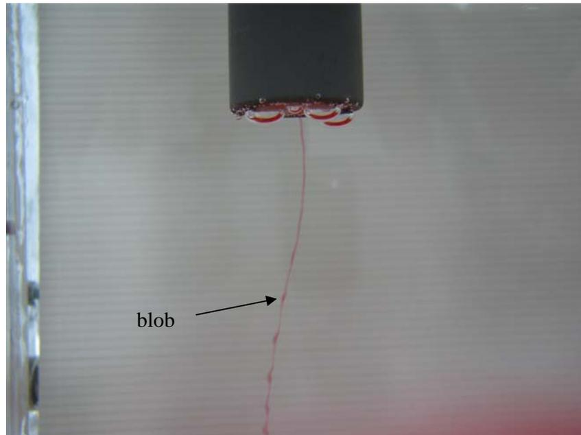
Figure 5 Blobs in the starting flow
