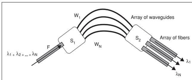
Fig. 2. Arrayed Waveguide Grating
