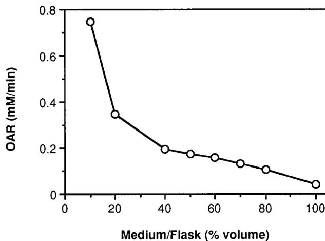
FIG. 1. Aeration efficiency (OAR) in shake flasks containing various volumes of culture medium (volume ratios in percentage of flask volume).
