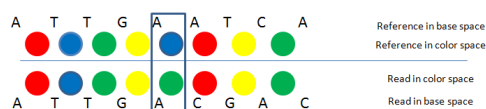
Fig. 1. Translating the read from color-space to base space may result in a new sequence different from the original read if there exists a base call error.
