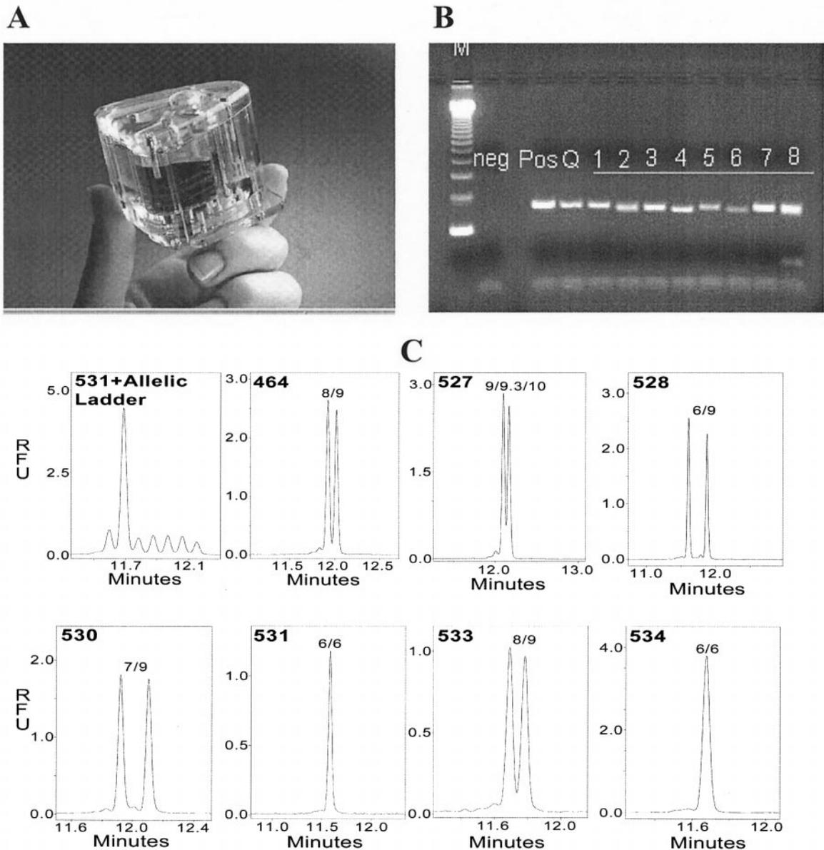
Fig. 1. Microfluidic cartridge for rapidly processing blood for PCR-based genetic testing (A), agarose gel electrophoresis of *TH01* STR PCR products (B), and STR polymorphism typing of the *TH01* locus using an automated sample preparation cartridge, the Smart Cycler PCR instrument, and the Beckman MDQ CE system (C).
