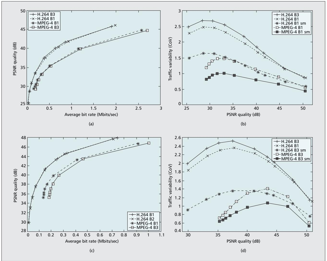
■ **Figure 3.** RD and VD graphs encoded with H.264/AVC “Full-RDO” and MPEG-4 Part 2 “ASP-Hpel” with GoP structures G16-B1 and G16-B3 without and with frame size smoothing (sm): a) RD graph for CIF Sony Demo sequence; b) VD graph for CIF Sony Demo sequence; c) RD graph for CIF Silence of the Lambs; d) VD graph for CIF Silence of the Lambs.
