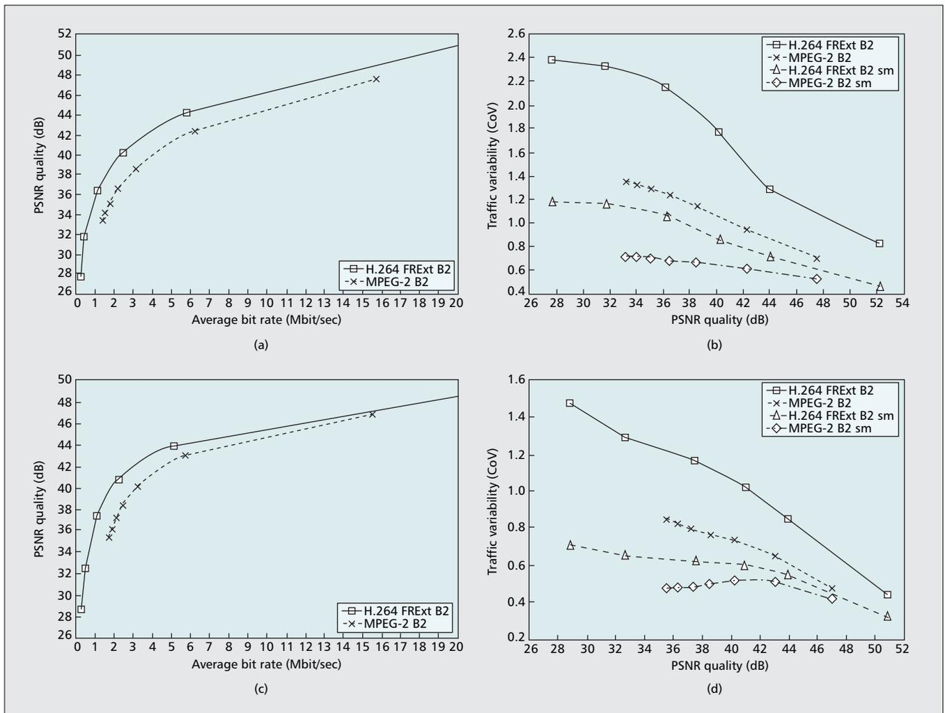
■ **Figure 5.** RD and VD graphs for two 10 min HD sequences encoded with H.264/AVC FRExt and MPEG-2 with and without smoothing: a) RD graph for Sony Demo; b) VD graph for Sony Demo; c) RD graph for Terminator 2; and d) VD graph for Terminator 2.
