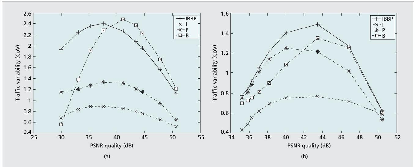
■ **Figure 2.** VD curves for I, P, and B frames, and overall sequence (IBBP), for Silence of the Lambs encoded with a) H.264/AVC “Full-RDO”; b) MPEG-4 Part 2 “ASP-Hpel.”
