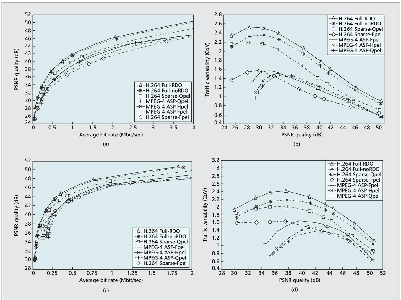
**Figure 1.** RD and rate VD characteristics for CIF Sony Demo and Silence of the Lambs encoded with H.264/AVC with and without new encoding tools and MPEG-4 Part 2 with range of pixel accuracy in MCP: a) RD graph for Sony Demo; b) VD graph for Sony Demo; c) RD graph for Silence of the Lambs; d) VD graph for Silence of the Lambs.
