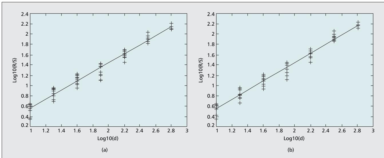
■ **Figure 4.** Pox diagrams of  $R/S$  with aggregation level  $a = 48$  for Silence of the Lambs  $G16-B3$  encodings: a) H.264/AVC,  $QP = 24$ ,  $H = 0.876$ ; b) MPEG-4 Part 2,  $q = 4$ ,  $H = 0.893$ .
