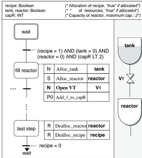
Figure 5: Structure of a recipe function block
