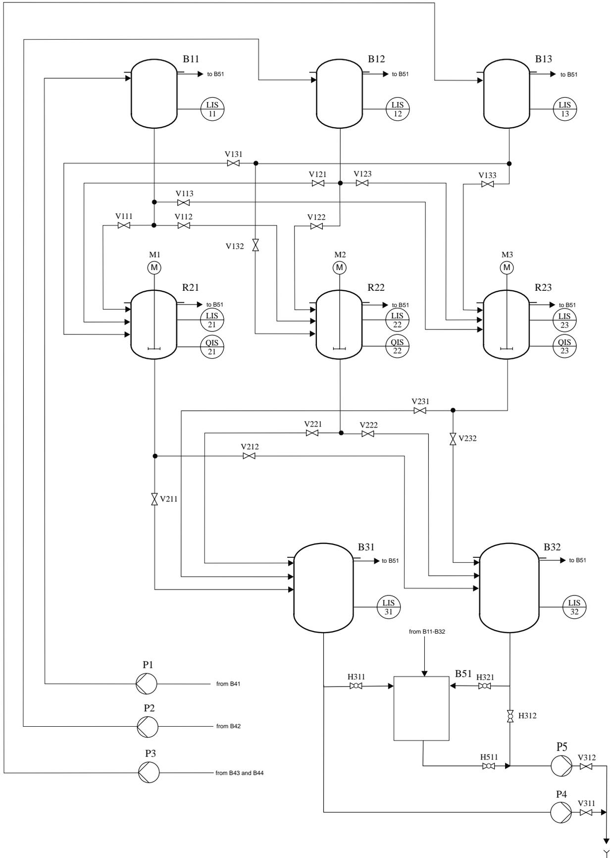
Figure 1: Piping and instrumentation diagram of the demonstration plant
