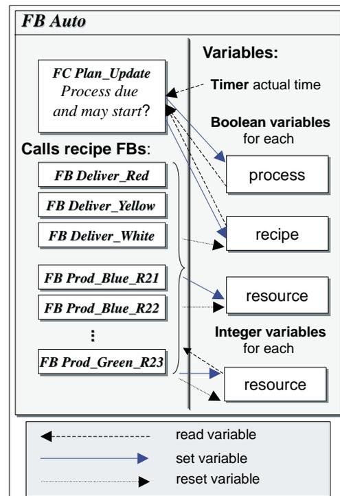
Figure 4: Structure of the automatic mode function block
