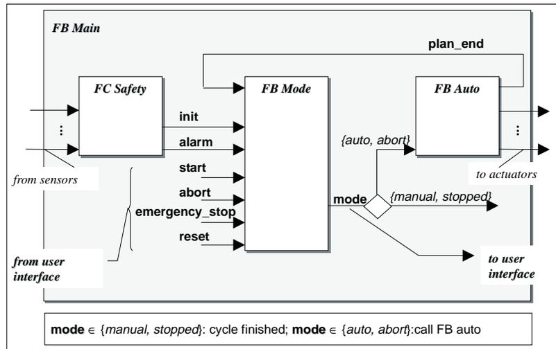
Figure 2: Top layer of the control program
