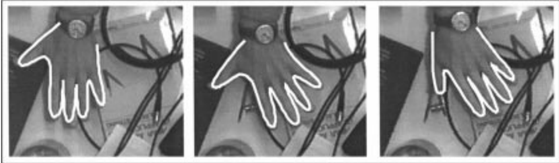
Figure 16. Tracking a flexing hand across a cluttered desk: representative stills from a 500 field (10 s) sequence show a hand moving over a highly cluttered desk scene. The fingers and thumb flex independently, and the hand translates and rotates. Here the CONDENSATION algorithm uses N = 1500 samples per time-step initially, dropping gradually over 4 fields to N = 500 for the tracking of the remainder of the sequence. The mean configuration of the contour is displayed.
