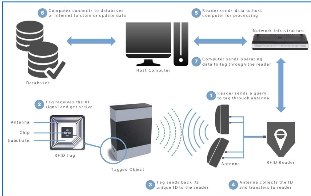
Figure 2: RFID Operation System
