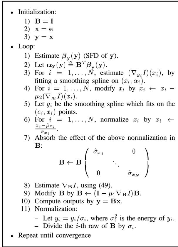
Fig. 7. The gradient approach for separating PNL mixtures.
