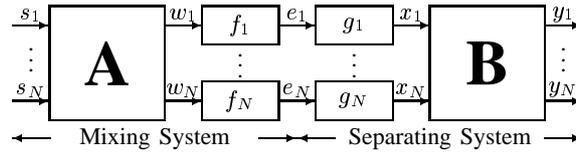
Fig. 2. The mixing-separating system for PNL mixtures.
