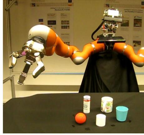
Fig. 3. The robot arm and gripper are used for manipulation, and Kinect is used to compute object features. Several objects are included while learning and verifying the planning capability in the real world.
