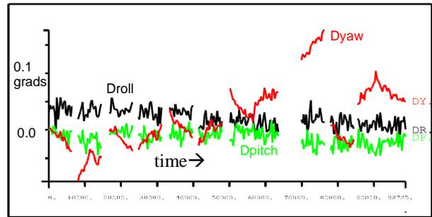
Figure 8: discrepancies of the attitude data corrected IMU – bundle block adjustment f(time)
