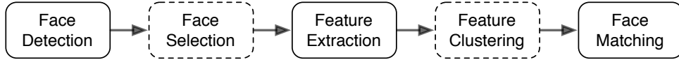
Figure 1: A recognition system with the proposed face selection and feature clustering steps highlighted.
