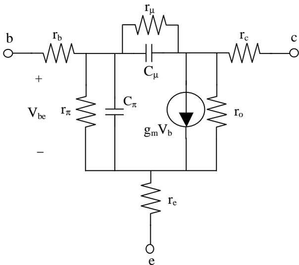
Fig. 1. Intrinsic high-frequency hybrid- $\pi$  model.
