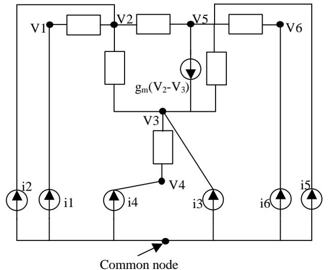
Fig. 2. Equivalent circuit for indefinite admittance matrix.
