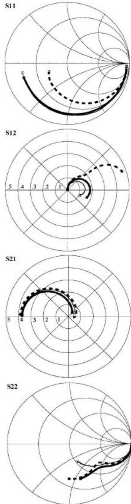
Fig. 5. Comparison of measured (light), calculated (bold), and simulated (dash)  $s$ -parameters for npn BJT at  $V_{CE} = 1V$  and  $I_C = 1mA$  from 45 MHz to 20.045 GHz.
