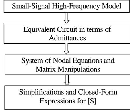
Fig. 3. Sequence of steps for derivation of closed-form expressions for s-parameters of BJTs.
