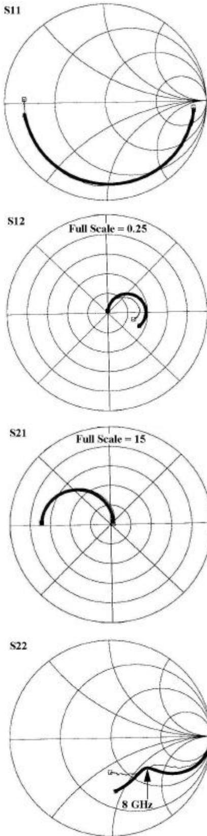
Fig. 4. Comparison of measured (light) and calculated (bold) s-parameters for npn BJT at  $V_{CE} = 3V$  and  $I_C = 3mA$  from 45 MHz to 20.045 GHz.
