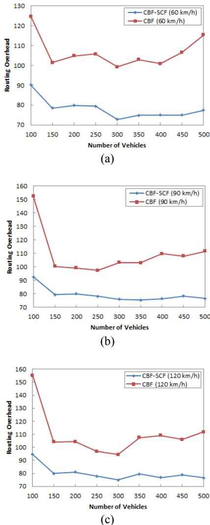
**Figure-8.** Routing overhead with different node speeds.
