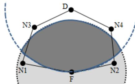
**Figure-1.** Forwarding node F is a local maximum with respect to destination D [24].
