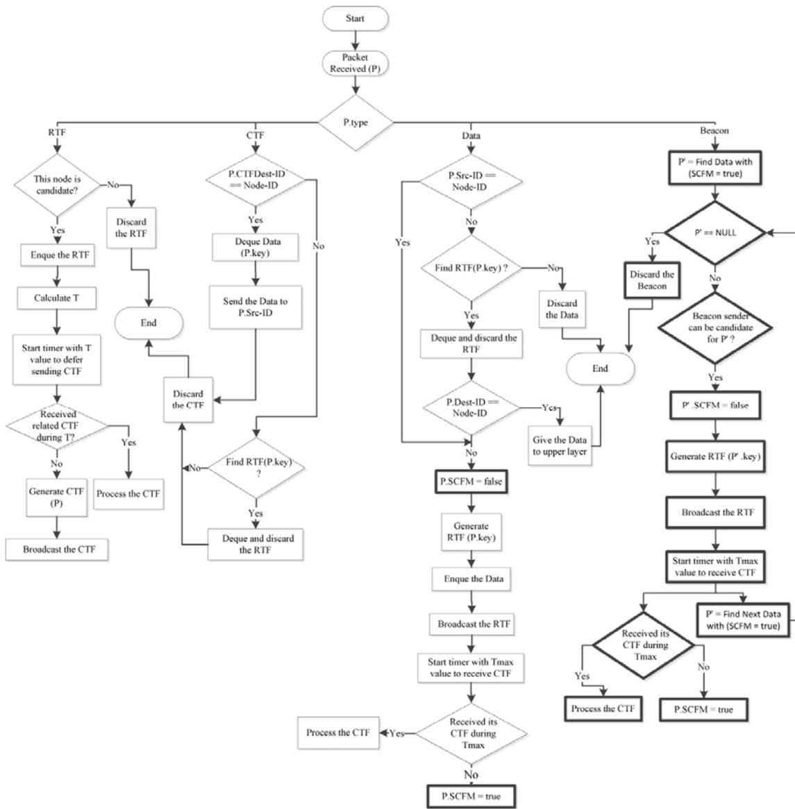
**Figure-4.** Flow chart of CBF-SCF protocol with relation between greedy mode (normal boxes) and SCF mode (bold boxes).
