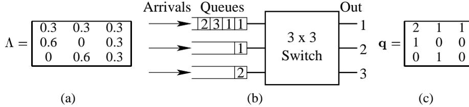
Figure 1: The packet arbitration model. (a) In each time slot, packet sources generate  $\lambda_{ij} \in \Lambda$  packets on average at input  $i$  for output  $j$ . (b) Packets arrive at an input queued switch and are stored in queues. The number indicate to which output the packet is destined. (c) The corresponding queue states, where  $q_{ij} \in \mathbf{q}$  indicates the number of packets waiting at input  $i$  destined for output  $j$ .
