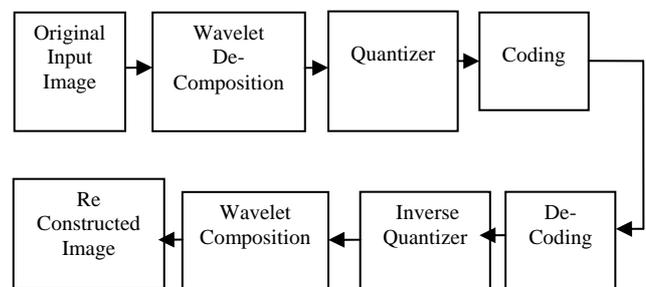
Figure 2. Block diagram of EZW image CODEC.
