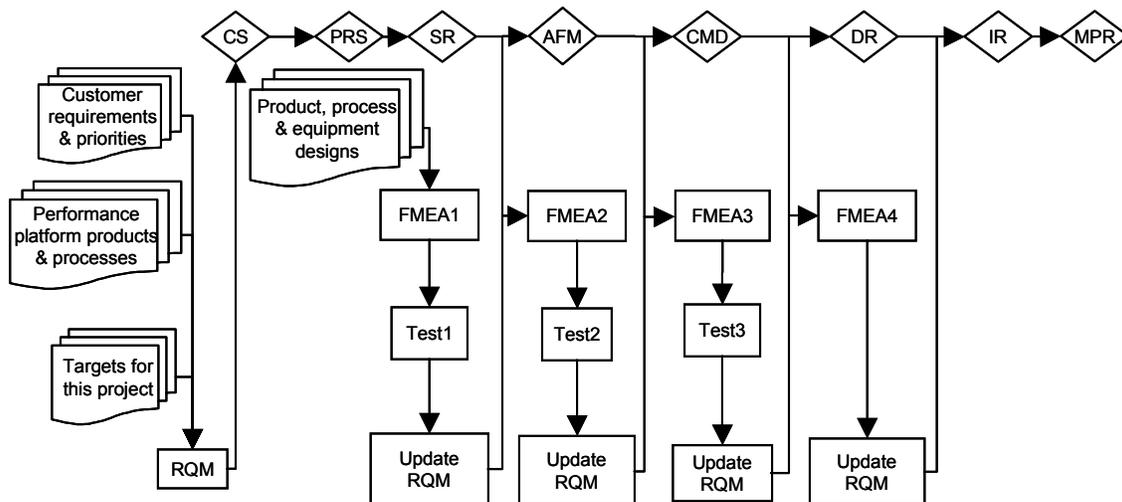
Figure 6.1 Proposal for implementation of RQM in the PDP
