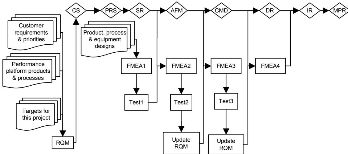
Figure 6.2 Actual implementation of RQM in the PDP
