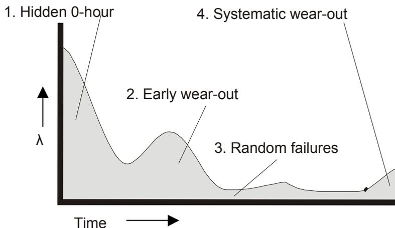
Figure 2.4 Four-phase roller-coaster reliability curve (Brombacher, 1992)
