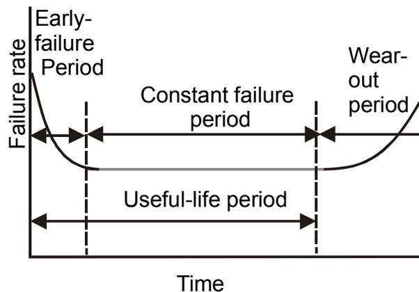
Figure 2.1 Bathtub failure rate curve
