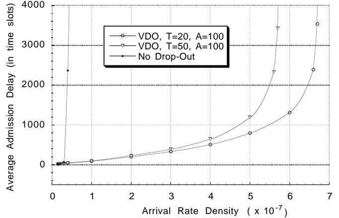
Figure 2: Average admission delay of a call (link) as a function of the arrival rate density  $\lambda_d$  for the cases of 1) voluntary drop-out (VDO) with  $T = 20 t.u.$  and  $A = 100 t.u.$ , 2) voluntary drop-out with  $T = 50 t.u.$  and  $A = 100 t.u.$ , and 3) no drop-out.
