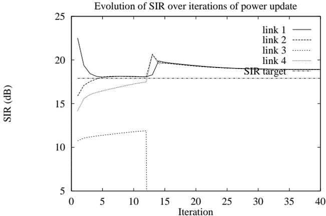
Figure 1: Evolution of the SIRs of the four mobile-to-base links under the DPC-ALP power control algorithm with SIR targets  $\gamma$  set 2dB above the SIR threshold achievable by all links.
