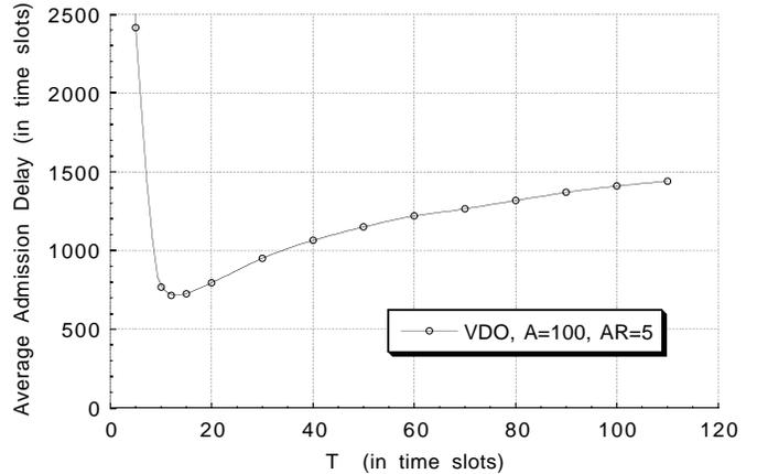
Figure 3: Average admission delay as a function of  $T$  for the case of voluntary drop-out (VDO) with  $A = 100 t.u.$  at fixed arrival rate (AR) density  $\lambda_d = 5 \times 10^{-7} \text{ arrivals}/(t.u. \times l.u.^2)$ .
