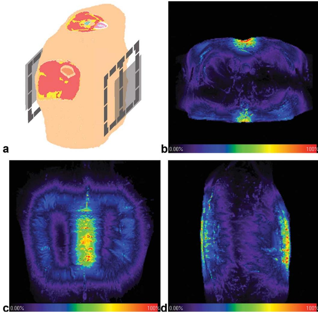
**Figure 3.** FDTD simulation setup with a truncated torso model (a). MIP of nonaveraged SAR distribution in a transversal (b), coronal (c), and sagittal (d) slice at 30W input power and best  $B_1^+$  shim phase setting. The RF power deposition is scaled from 0 (black) to 42 W/kg (red), the corresponding maximum 10 g averaged SAR is 15.1 W/kg, partial body SAR is 1.4 W/kg.
