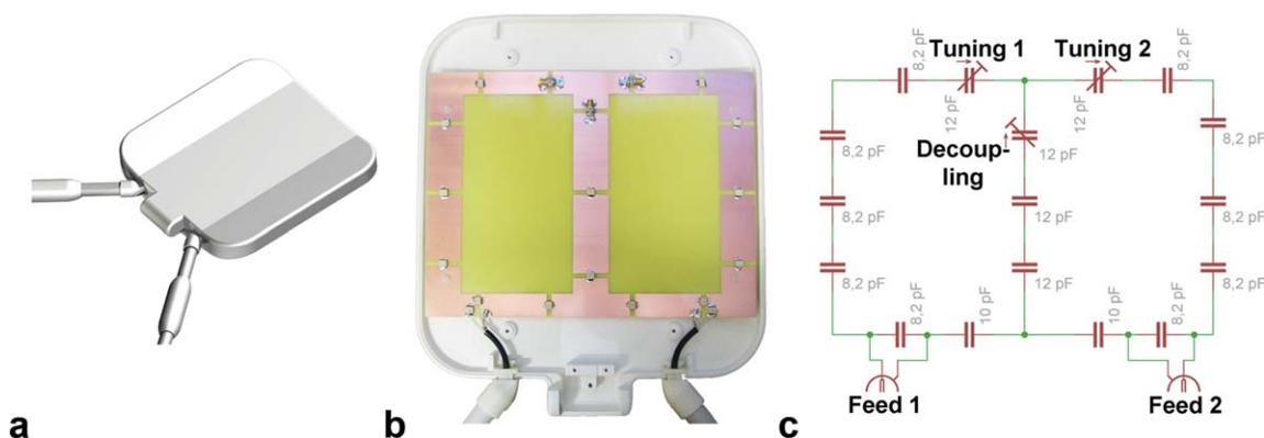
**Figure 1.** A rendered 3D model of one modestly curved lightweight coil casing former (a) together with the interior of the proposed coil design (b) and the basic circuit diagram (c). [Color figure can be viewed in the online issue, which is available at [wileyonlinelibrary.com](http://wileyonlinelibrary.com).]
