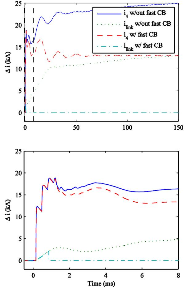
Figure 5. Fault current contribution from mirrored subsystem,  $i_{link}$ , to the fault current  $i_4$  with and without a fast CB at location of  $i_{link}$ .
