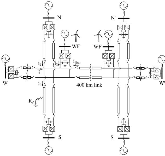
Figure 4. Modified system for investigation of selective placing of CBs.
