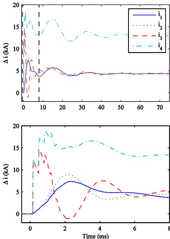
Figure 2. Short circuit currents in for pole-to-ground fault in four-terminal test system using base case parameters.
