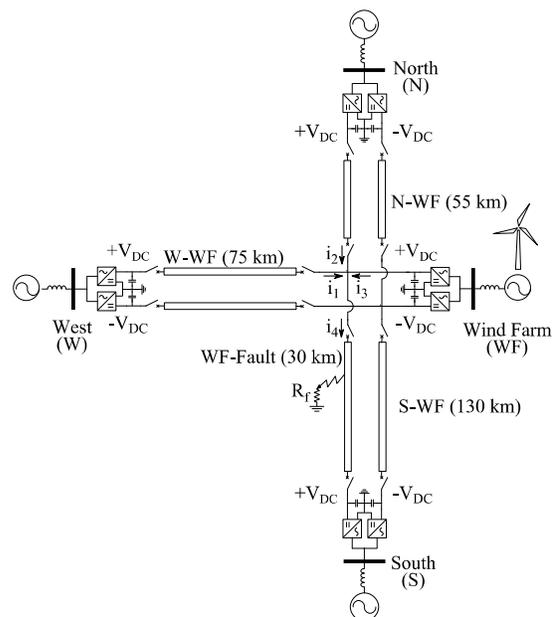
Figure 1. Four-terminal VSC-HVDC test system.
