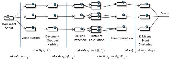
Figure 3. Event Detection using sub-stream partitioning in Storm.
