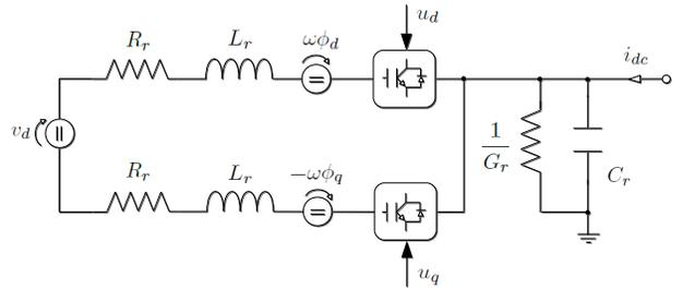
Fig. 2. Schematic diagram of the equivalent circuit of a VSR in  $dq$  frame.
