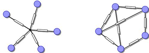
Fig. 1. Nodal representation of HVDC transmission systems with radial and meshed topologies.
