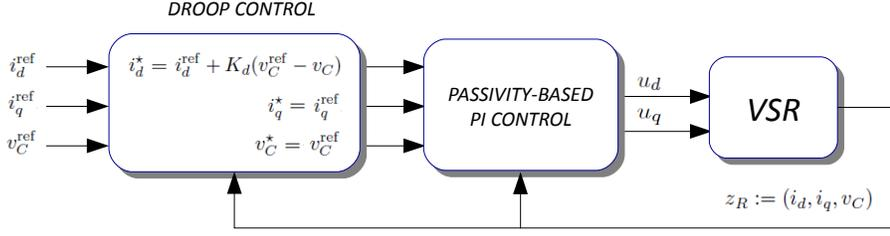
Fig. 7. Closed-loop representation of the inner-loop PI-PBC plus the primary droop controller.
