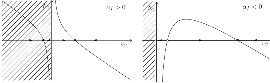
Fig. 3. Plot of  $\dot{v}_C$  versus  $v_C$  for the cases of (a)  $\alpha_I > 0$  and (b)  $\alpha_I < 0$ . The arrows in the horizontal axis indicate the direction of the flow.
