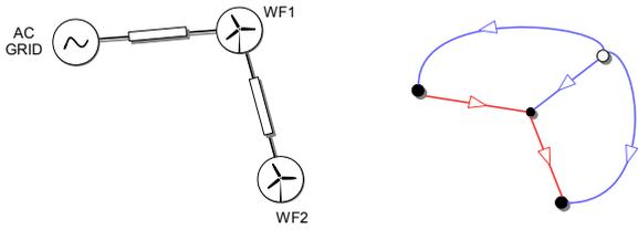
Fig. 4. Schematic representation of an HVDC transmission system constituted by three stations, associated to two wind farms (WFs) and an AC grid, with associated graph. The graph is represented by filled circles for the *VSRs-buses* and the unfilled circle for the *ground* node. Blue and red edges characterize VSRs and lines, respectively.
