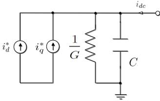
Fig. 8. VSR modeled as ideal current sources connected to a voltage bus capacitor, in  $dq$ -frame.
