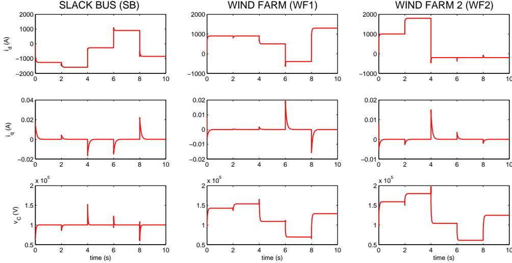
Fig. 9. Responses of VSRs variables with the decentralized PI-PBC plus droop control.
