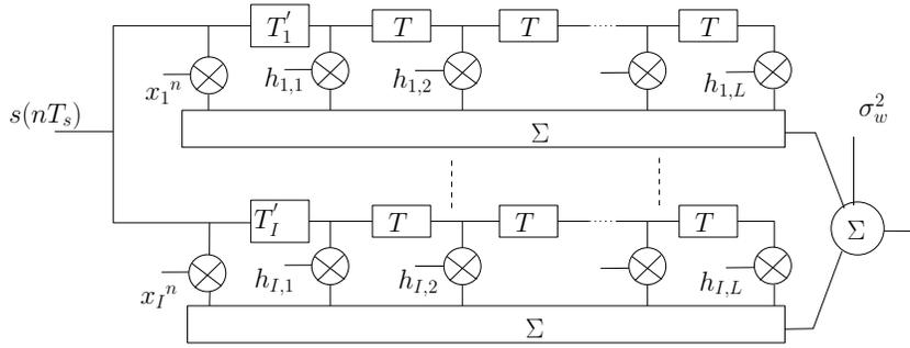
Fig. 6. Composite channel response capturing CFO / doppler spread, propagation delay differences, as well as multi-path reflections.
