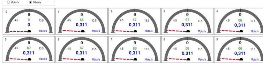
(b) A screenshot of the GUI's speedmeter. Real-time streaming from 9 nodes towards the sink, showing a sustained throughput of 310 kbps for all streaming nodes.
