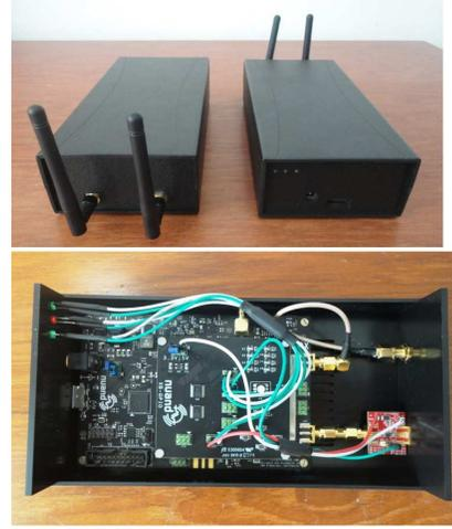
Fig. 4. An SDR platform from Nuand was used to build the contention-free geo-routing protocol.
