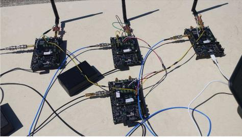
Fig. 8. Common clock and trigger signals are fed into the boards. The controlled test setup is used to measure the performance of the decision-directed equalization method.
