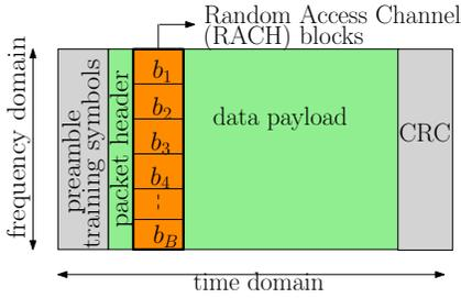
Fig. 1. A random access channel is inserted into the OFDM frame to allow concurrent transmitters to stamp their position information.
