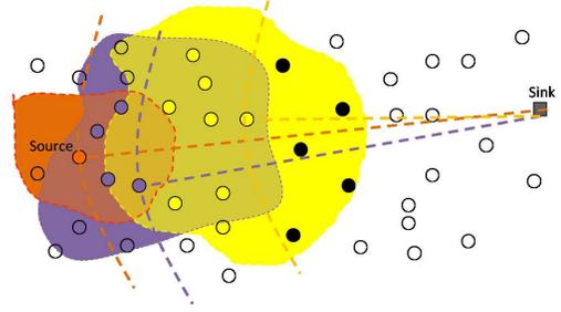
Fig. 2. Illustration of the operation of the contention-free geo-routing scheme. A source injects a frame into the network. Receivers who are closer to the sink than the source relay the frame. In the second hop, each receiver goes through position information conveyed by the transmitters of the first hop to decide whether to forward the frame or not. Any second-hop receiver which offers positive progress towards the sink will decide to forward.
