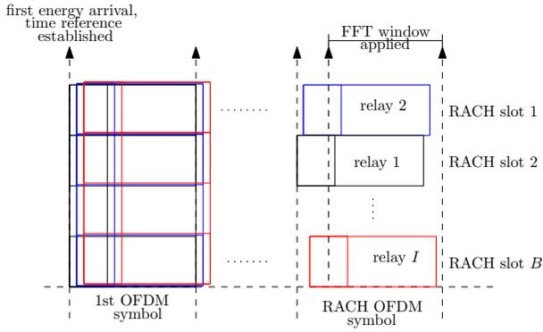
Fig. 5. Illustration of the time offset problem on the RACH portion of the frame.
