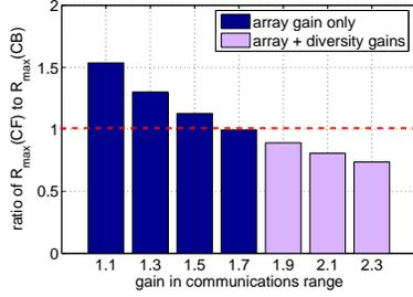
Fig. 3. The maximum achievable throughput per node for the case of contention-free divided by that of contention-based geo-routing. The computation was carried out assuming a network of 40 nodes at a density of  $\rho = \frac{1}{82} \text{m}^{-2}$ . The communication range was  $\leq 25\text{m}$  at a path loss coefficient of 2.8. Packet duration of 1ms at an arrival rate of  $30\text{s}^{-1}$ .
