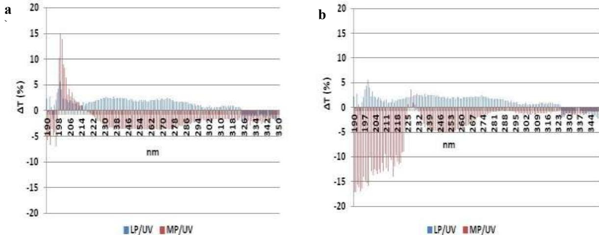
Figure 2. Transmittance variability ( $T_{(before\ UV)} - T_{(after\ UV)} / T_{(before\ UV)}$ ), in percentage, of the wastewater before UV radiation and after LP/UV or MP/UV radiation related to the wastewater before UV radiation). (a) WWTP 1 and (b) WWTP 2.
