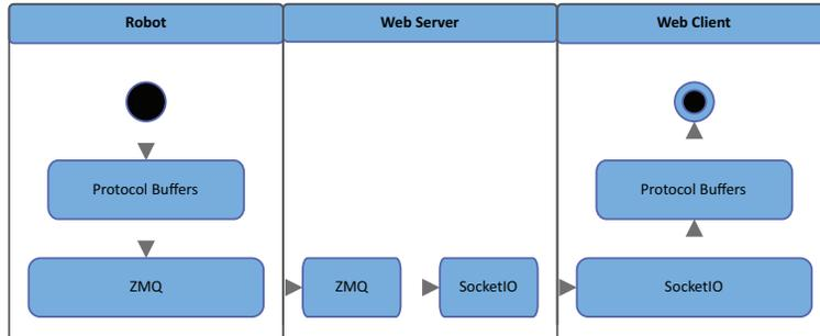
**Fig. 2.** Visual representation of the flow of information between the various networking packages implemented during the development of NUbugger. The selected libraries provide sufficient levels of abstraction over underlying network communication that the robots and web clients need not be coded in the same language.
