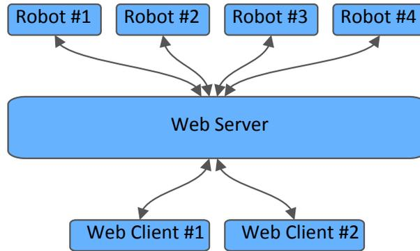
**Fig. 1.** Visual representation of the many-to-many NUbagger implementation, allowing multiple users to visualise the real-time performance of an arbitrary number of robots. The selected libraries provide sufficient levels of abstraction over underlying network communication that the robots and web clients need not be coded in the same language.
