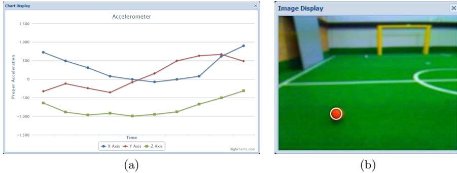
**Fig. 4.** Two examples of NUbagger debugging interfaces: a) the scrolling chart display, demonstrating real-time information from the robot’s 3-axis accelerometer; and b) the image display, with an overlay demonstrating the correct identification of the ball [2].
