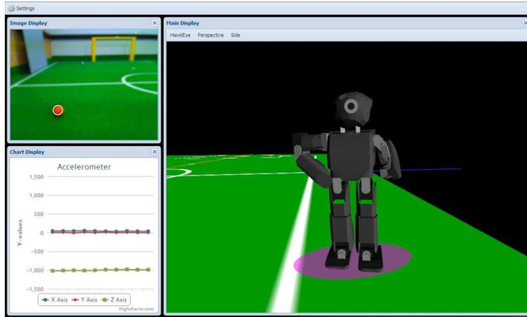
**Fig. 3.** The NUBots configuration of the NUbugger utility, demonstrating: the main display (right), image display (top-right) and scrolling chart display (bottom-left). These displays are able to be customised by the user to provide any manner of real-time information from the robot.
