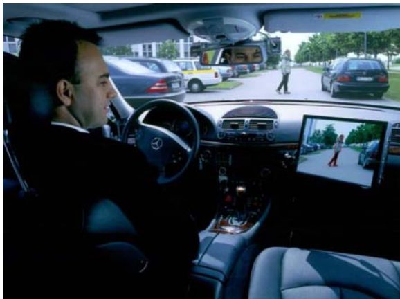
Figure 10. Inside the vehicle demonstrator: stereo cameras visible lateral to rear-mirror, display for system prototyping.
