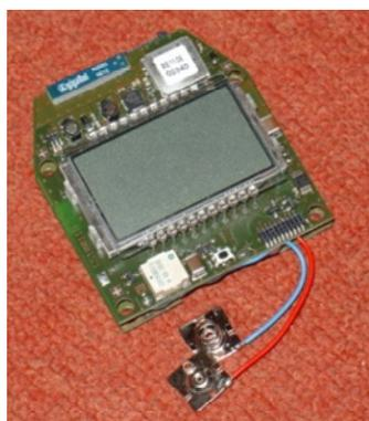
Figure 4 12 channel ECG bluetooth module BlueECG
