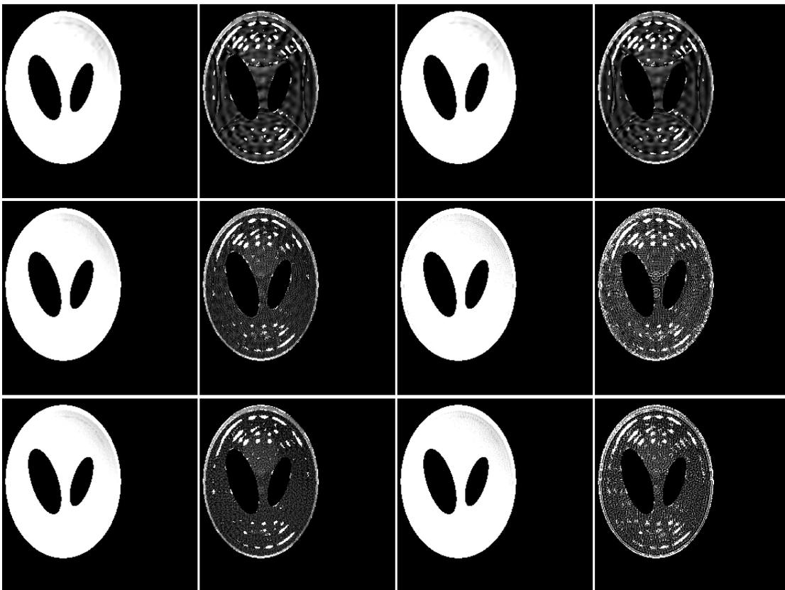
Fig. 5. Reconstruction of Phantom image. 1<sup>st</sup> row – Uniform under-sampling, 2<sup>nd</sup> row – Radial sampling, 3<sup>rd</sup> Row – Gaussian under-sampling; 1<sup>st</sup> Column – SparSENSE reconstructed image, 2<sup>nd</sup> Column – SparSENSE reconstructed difference image, 3<sup>rd</sup> Column – proposed NN regularized SENSE reconstructed image; 4<sup>th</sup> Column - proposed NN regularized SENSE reconstructed difference image.
