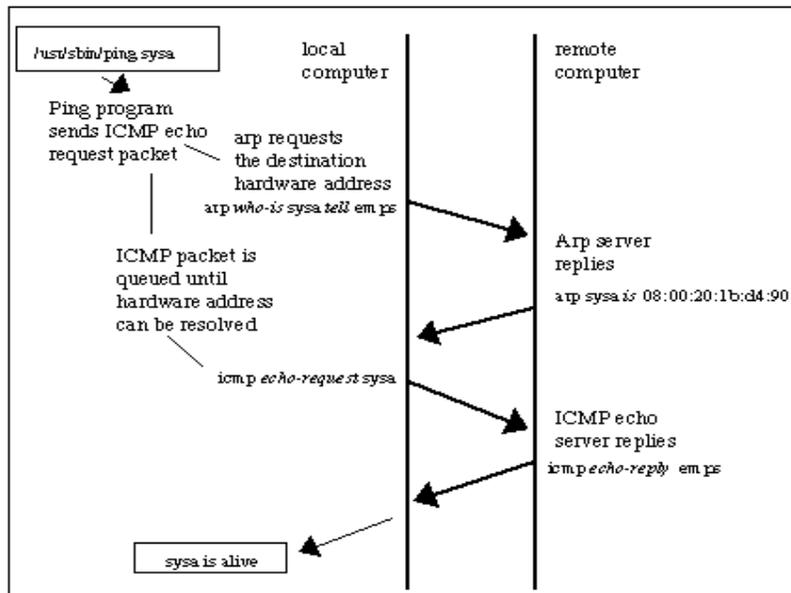
**Figure 1. Typical ARP packet exchange. From [7]**
