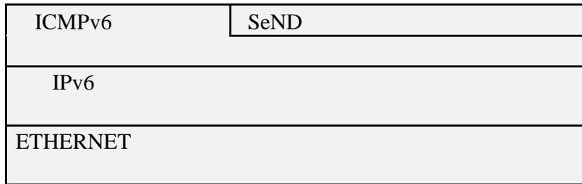
**Figure 3. Logical placement of SeND in IPv6.**
