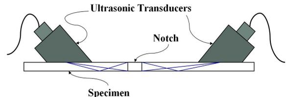
Fig. 2. Ultrasonic Flaw Detection scheme
