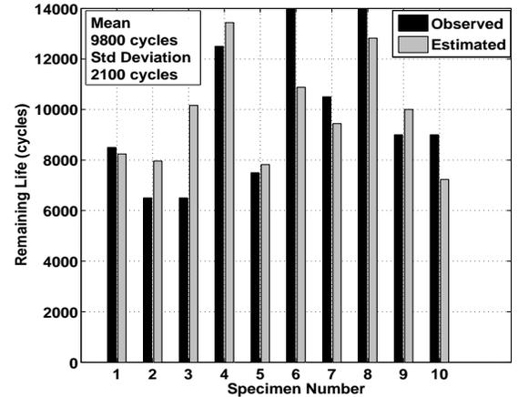
Fig. 6. Observed and Estimated Remaining Life after curvature threshold is crossed for 10 samples
