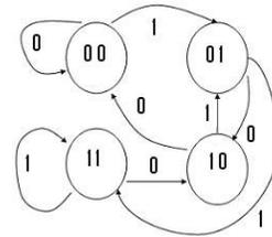
Fig. 3. Finite state automaton with  $D = 2$  and  $\mathcal{A} = \{0, 1\}$
