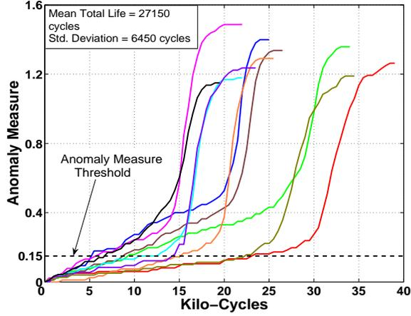
Fig. 4. Anomaly Measure plots for Stochastic Data of 10 similar specimens under identical loading
