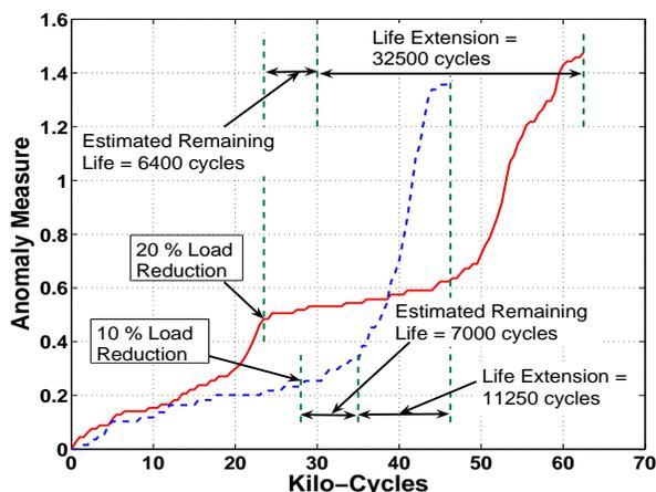
Fig. 7. Realtime Life Extension for two experiments with different levels of load reduction
