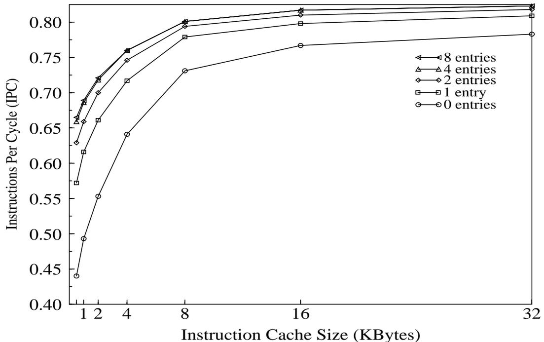
Fig. 4: Stream buffer compensating for reduced instruction cache size.
