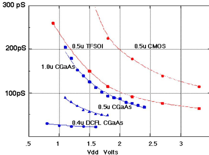
Fig. 2: Propagation delay of CGaAs, CMOS, and TFSOI versus supply voltage [2].
