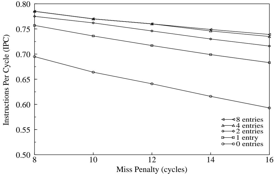
Fig. 5: Stream buffer compensating for increased memory latency.
