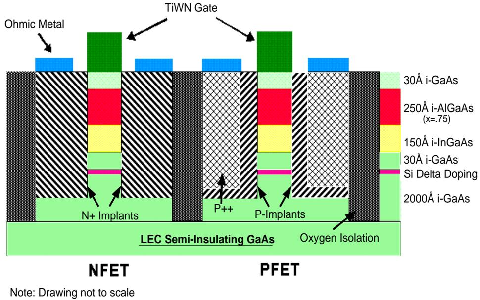
Fig. 1: CGaAs process cross-section [2].
