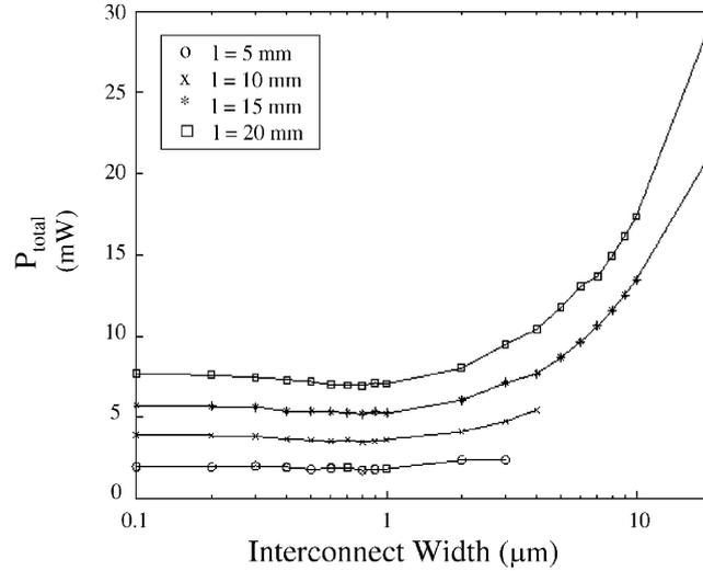
Fig. 9. Total transient power dissipation as a function of interconnect width.
