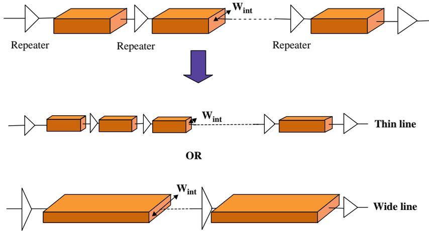
Fig. 3. Wire sizing in a repeater insertion system.
