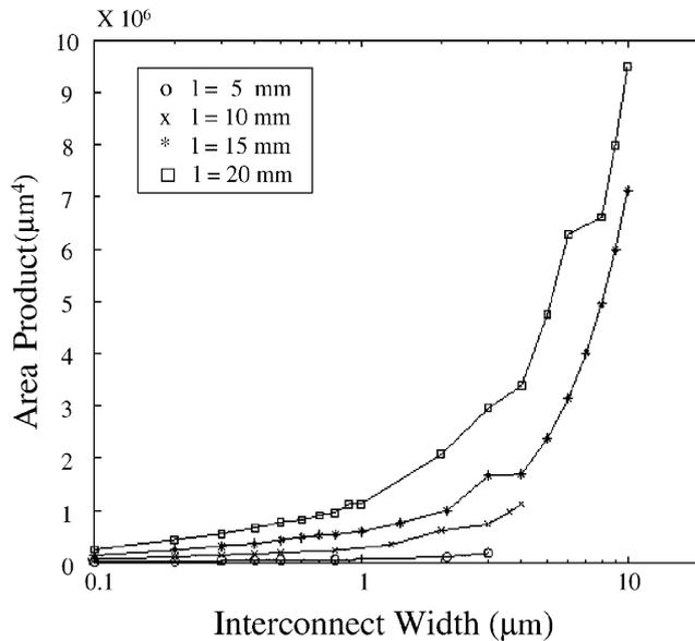
Fig. 12. Product of interconnect and transistor area as a function of the interconnect width for different line lengths.
