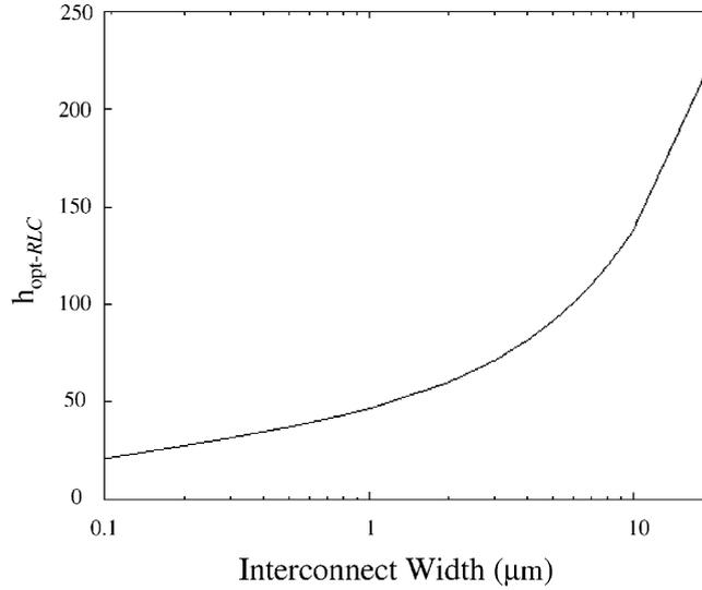
Fig. 5. Optimum repeater size for minimum propagation delay for different line widths.
