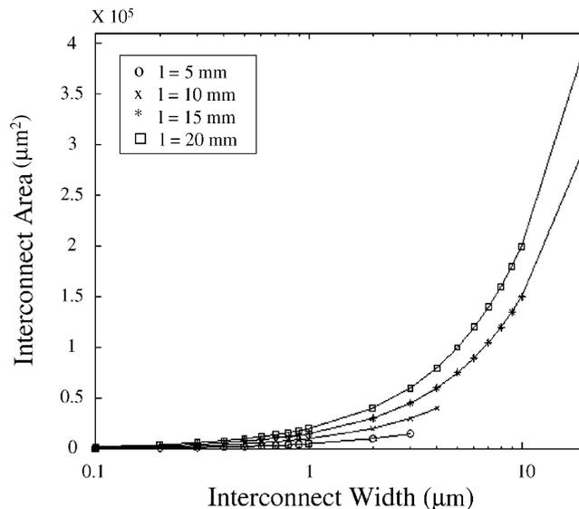
Fig. 10. Interconnect area as a function of interconnect width for different line lengths.
