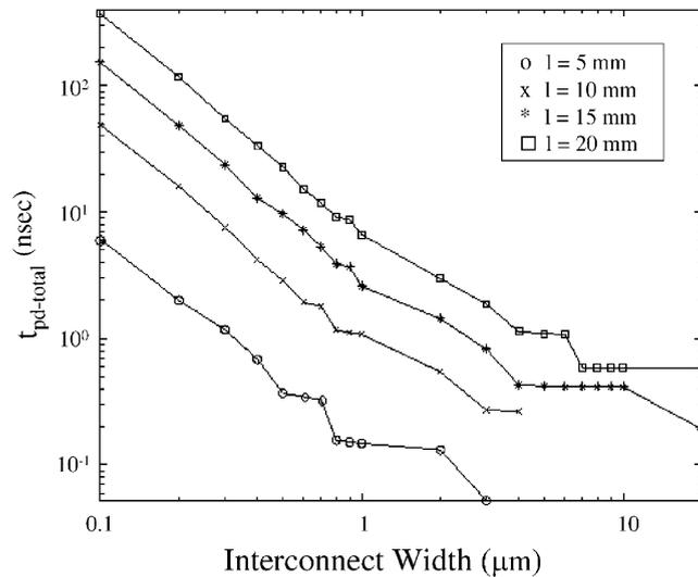
Fig. 7. Minimum signal delay as a function of interconnect width for different line lengths.
