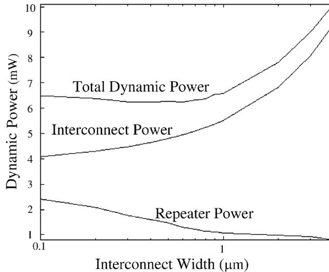
Fig. 8. Dynamic power dissipation as a function of interconnect width for  $l=20$  mm.
