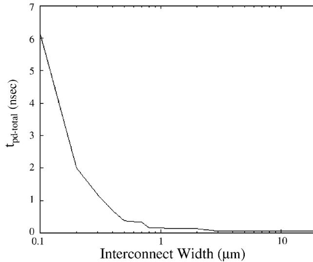
Fig. 6. Minimum signal propagation delay as a function of interconnect width ( $l = 5$  mm).
