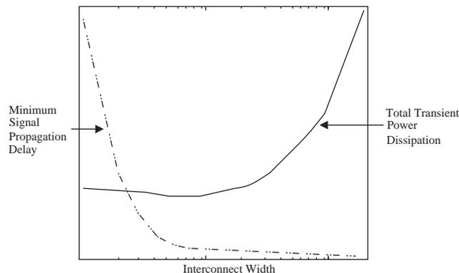
Fig. 1. Minimum signal propagation delay and transient power dissipation as a function of line width for a repeater system.
