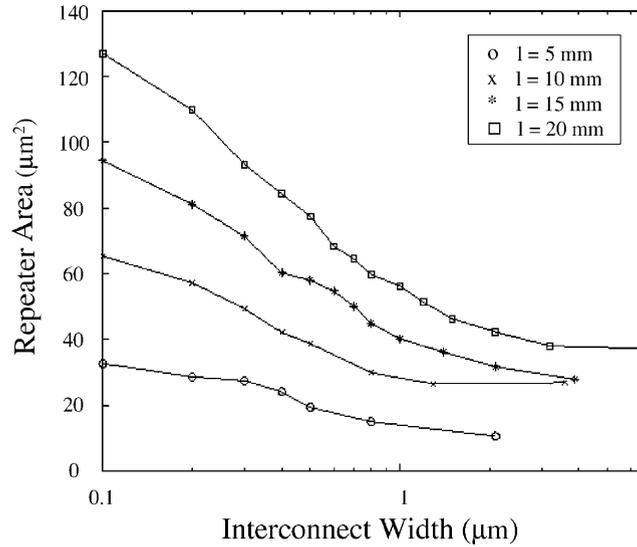
Fig. 11. Total area of the repeaters as a function of the interconnect width for different line lengths.
