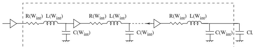
Fig. 2. Uniform repeater system driving a distributed  $RLC$  interconnect.
