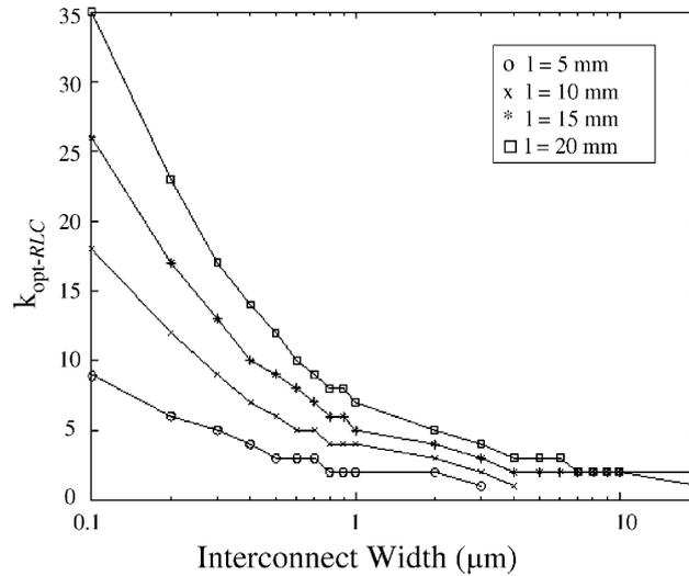
Fig. 4. Optimum number of repeaters for minimum propagation delay for different line widths.
