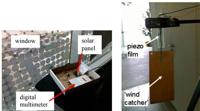
(a) Solar energy is harvested near a window in a typical office building. (b) PZ energy is produced when wind blows a “wind catcher” that bends the PZ material.
