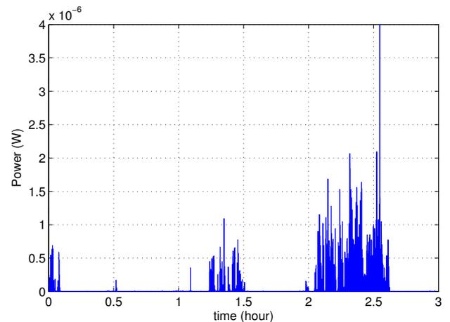
Fig. 1. Harvested PZ energy generated from natural wind over two hours.
