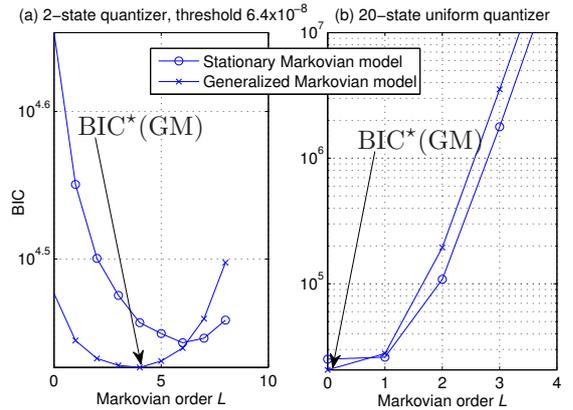
Fig. 4. BIC for harvested PZ energy. Different quantizer for  $E_k$  is used, while  $S_k$  is always quantized into two states with quantizer threshold  $2 \times 10^{-8}$ . Here, the minimum BIC is obtained with the GM model.
