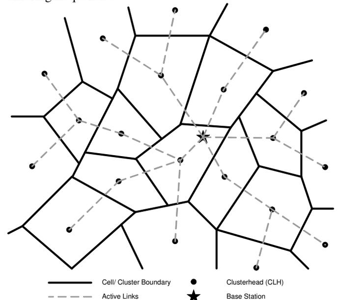
Figure 1. A tessellated or clustered wireless sensor network.
