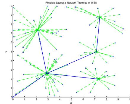
Figure 4. Physical layout & network topology of WSN
