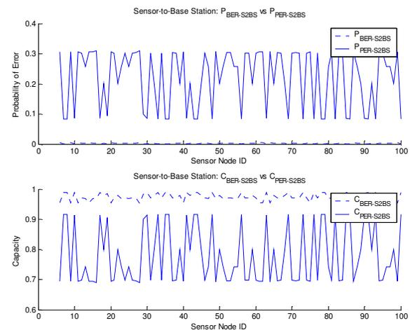
Figure 5. a) Sensor-to-Base Station Probability of Error for BER and PER, b) Sensor-to-Base Station channel capacity for BER and PER.
