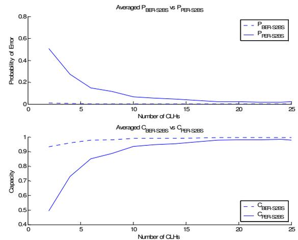
Figure 6. a) Sensor-to-base station channel capacity against number of clusters, averaged over 20 simulations.
