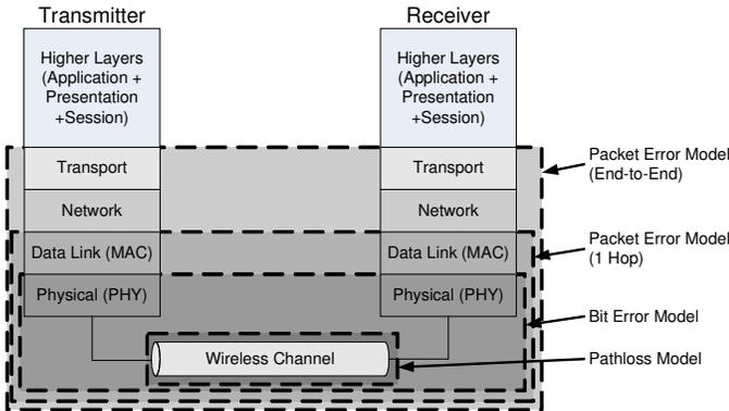
Figure 2. End-to-End channel between a transmitter and receiver on a multihop wireless network.
