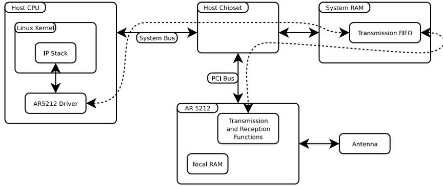
Figure 8: System architecture of an AR 5212-based device.
