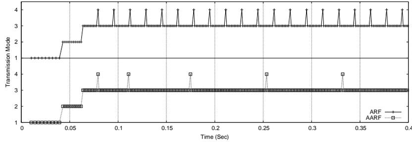
Figure 1: Mode selection comparison between ARF and AARF.
