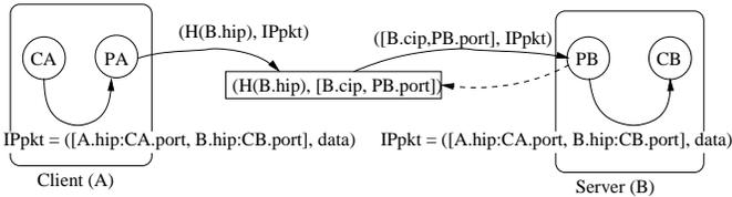
Figure 6: Legacy application support.  $A.hip$  and  $B.hip$  represents home IP addresses of hosts  $A$ , and  $B$ , respectively. Each host has a proxy that intercepts applications packets and send them via  $i3$ .
