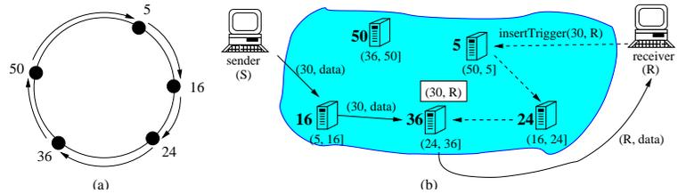
Figure 2: (a) A Chord identifier circle for  $m = 6$ , with 5 servers identified by 5, 16, 24, 36, and 50, respectively. (b) Receiver *R* inserting trigger ( $30, R$ ), and sender *S* sending packet ( $30, data$ ).
