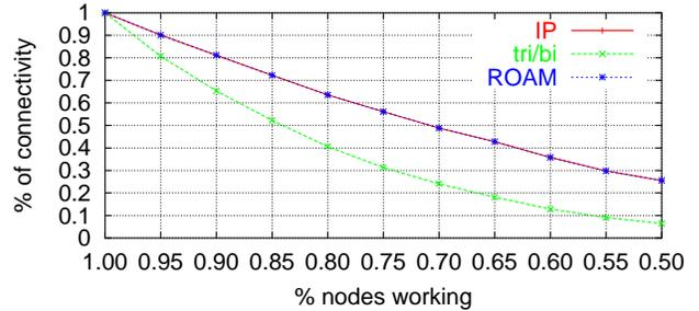
Figure 13: The robustness of IP, MIP (“tri/bi”), and ROAM. The  $x$ -axis shows the probability that an end host, home agent, or  $i3$  server is operational. The  $y$ -axis shows the probability that the CH and MH can communicate.
