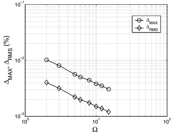
Fig. 5. Normalized maximum and RMS errors on  $\Gamma_o$  versus oversampling factor  $\Omega$ .
