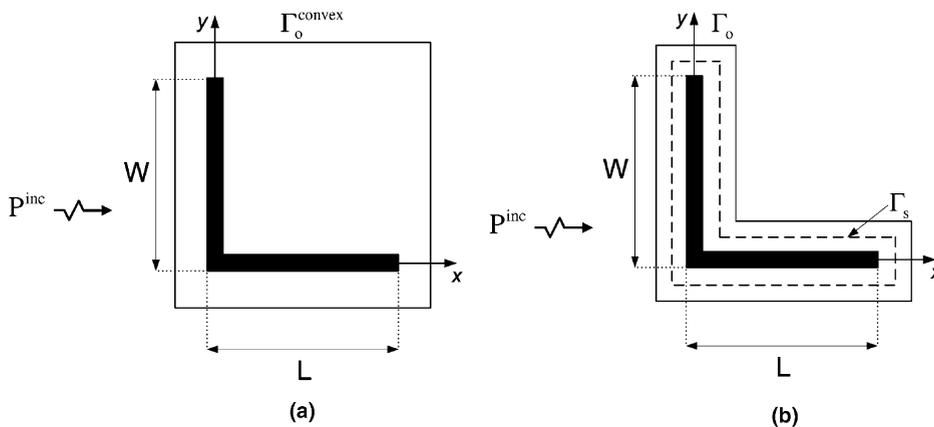
Fig. 4. L-shaped obstacle enclosed in: (a) convex computational domain, (b) conformal computational domain.
