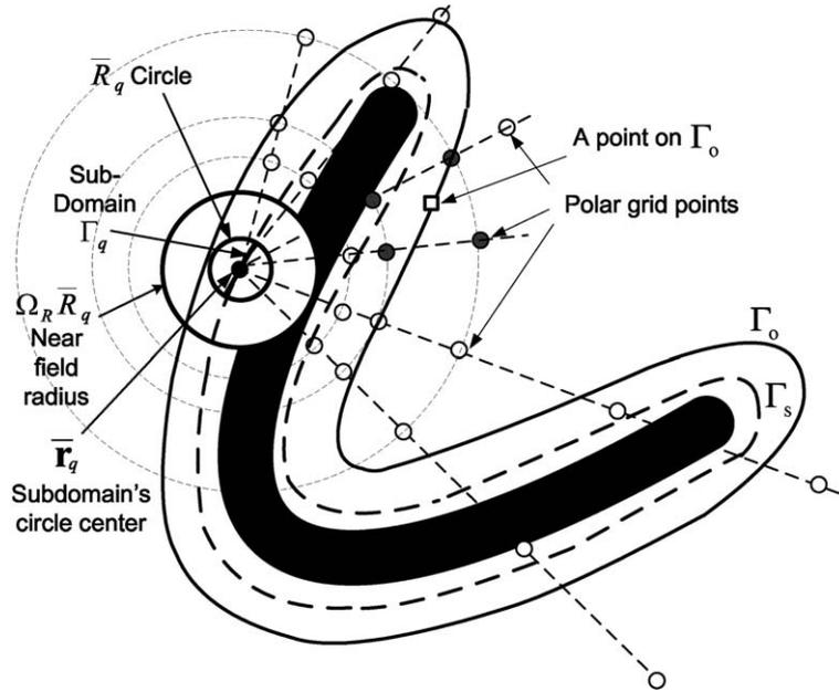
Fig. 3. A portion of the non-uniform polar grid (NG) for a selected subdomain and four NG points (shown as solid circles) used in the bilinear interpolation for a particular point on  $\Gamma_o$ .
