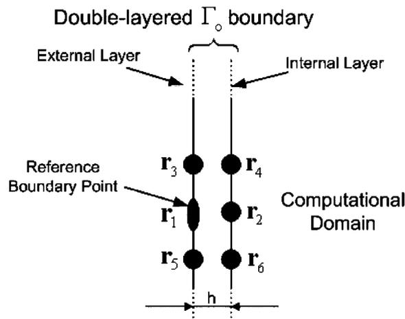
Fig. 2. Six-point stencil of Mur ABC on a double layered boundary.
