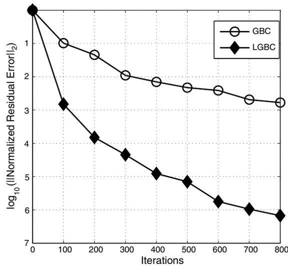
Fig. 9. Convergence rates of the GMRES algorithm for the LGBC in comparison to a GBC with Kirchoff-like integration of equivalent sources on  $\Gamma_s$ , resulting in the field on  $\Gamma_o$ .
