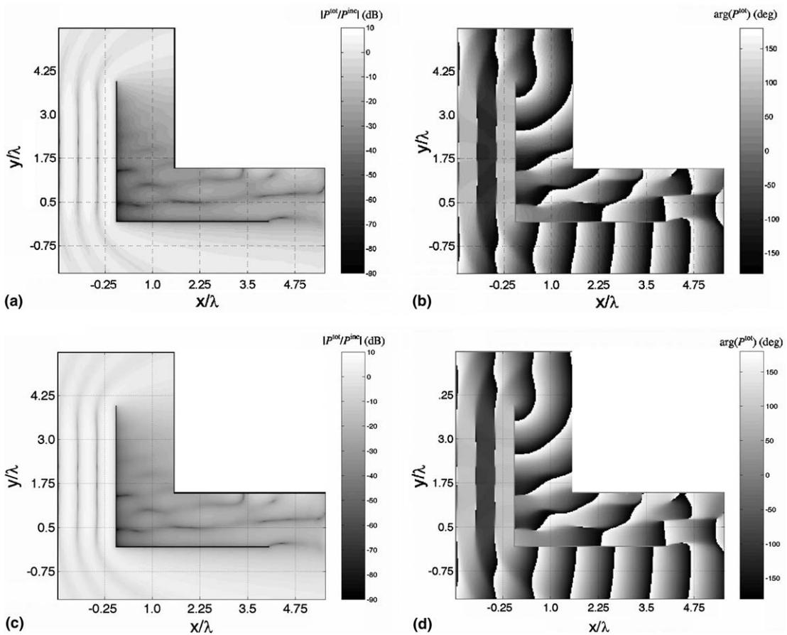
Fig. 6. Total acoustic pressure computed using LGBC via (I) direct integration: (a) amplitude; (b) phase, and (II) NG: (c) amplitude; (d) phase.
