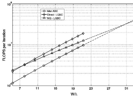
Fig. 8. Computational cost of various boundary conditions versus obstacle size in wavelengths.
