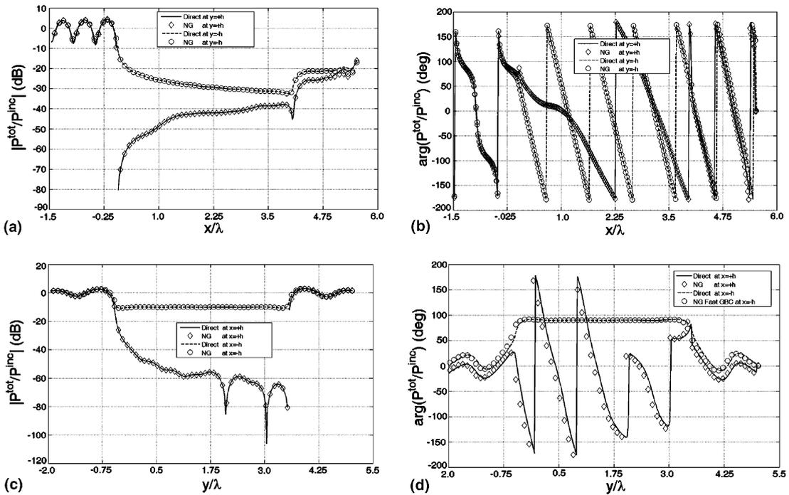
Fig. 7. Total acoustic pressure computed using direct and NG integrations LGBC: (a) amplitude versus  $x$ ; (b) phase versus  $x$ ; (c) amplitude versus  $y$ ; (d) phase versus  $y$ .
