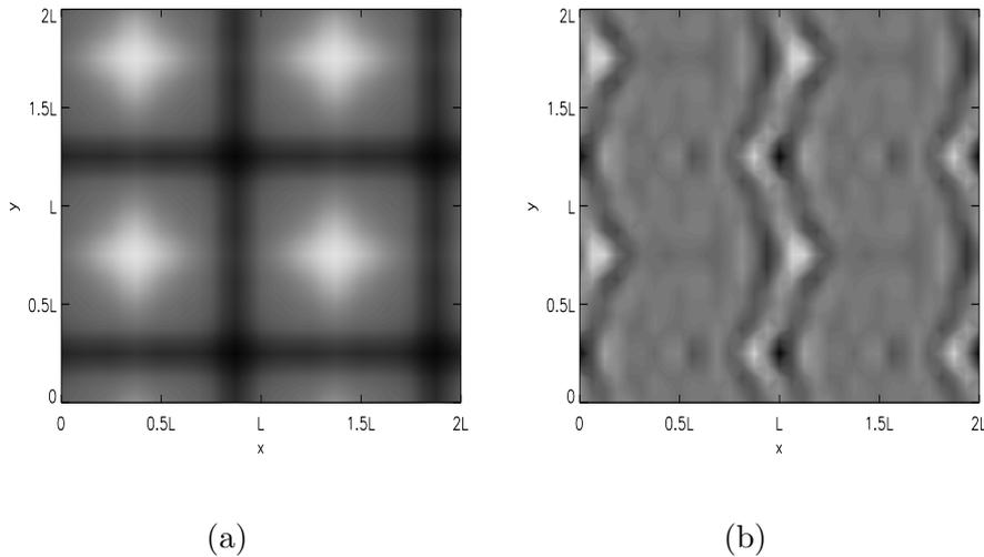
Fig. 4. Shadowgraph images of the vertical velocity component  $v_z$  of an asymmetric square pattern for  $R_a = 7000$  and  $T = 0$  (a) and of the vertical component  $B_z$  of the associated unstable magnetic eigenmode for  $P_m = 5.5$  (b). The values in the horizontal midplane are shown, bright areas indicating positive values.
