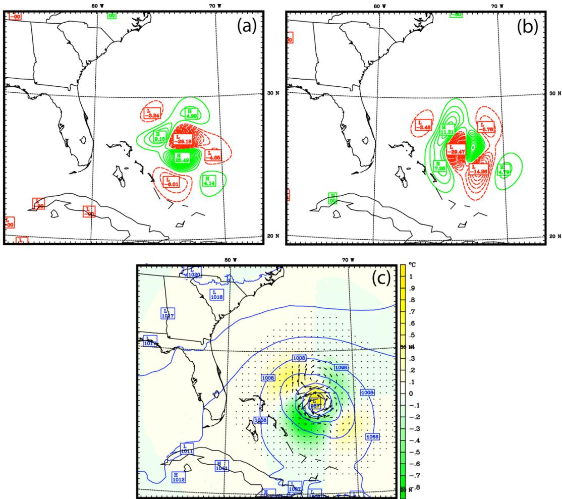
Figure 4: Increments of the ADR data assimilation experiment for Hurricane Jeanne (2004): (a) u increments, (b) v increments at 850 hPa, and (c) T increments at 300 hPa
