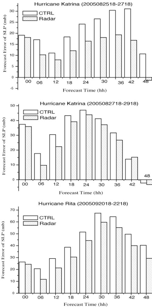
Figure 7: Forecasted hurricane intensity errors for each case (The white bar represents CTRL, and the gray bar is the one with assimilating ADR data)
