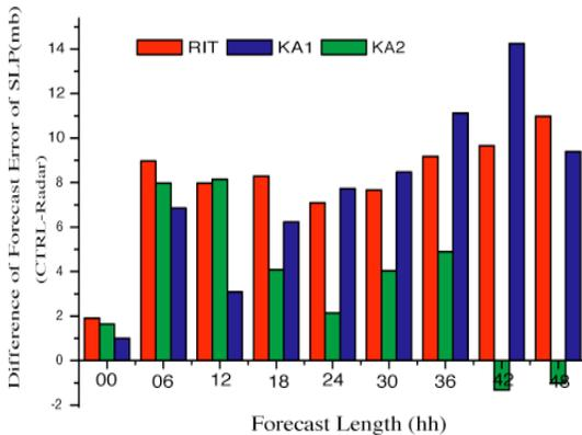
Figure 8: The difference of predicted intensity errors between CTRL and with radar data assimilation
