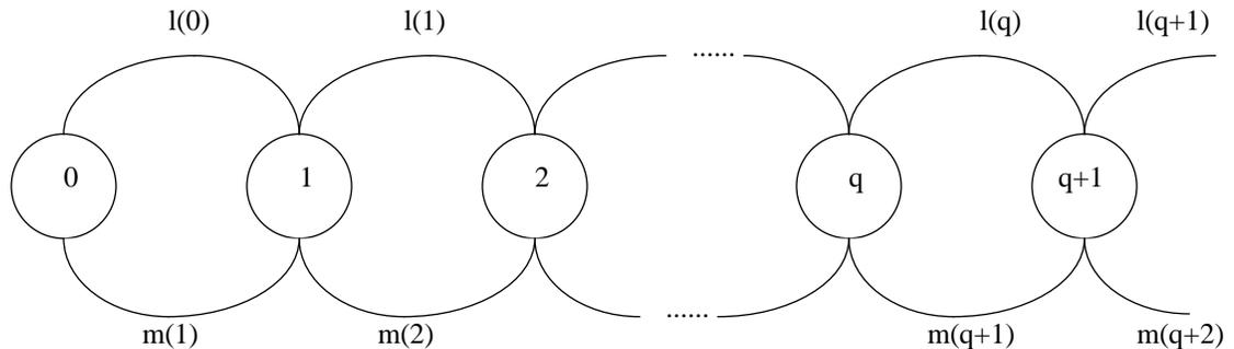
In the specific case of Almes' and Lazowska's application of this model, they used the approximate capacity formula for Ethernet of Metcalfe and Boggs [2] to determine the death rate. The assumption there was that with  $Q$  active users, the network would alternate between "contention periods" (similar to optimally controlled finite population slotted Aloha) and "packet transmissions". Under these assumptions, Metcalfe and Boggs found that the utilization is given by
