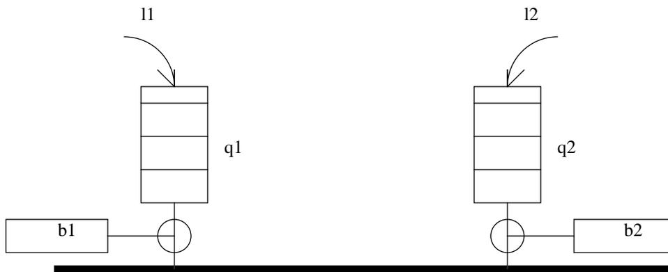
There are two stations attached to a network. Their state is characterized with number of packets in a queue and the backoff counter contents. They are denoted by  $q1$ ,  $q2$ ,  $b1$  and  $b2$ , respectively. The input to the stations is modelled by Poisson processes, with parameters  $l1$  and  $l2$ .
