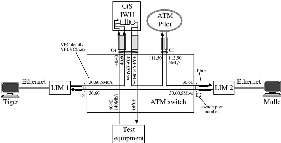
Figure 7 Experimental configuration with background traffic
