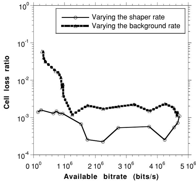
Graph 7 Effect of varying the shaper rate and background rate on the cell loss ratio
