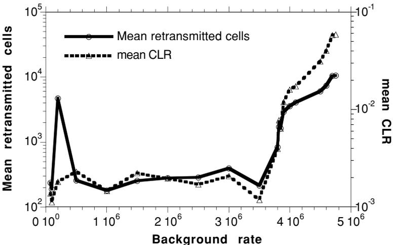
Graph 5 Retransmission overhead and cell loss ratio for background load experiment.
