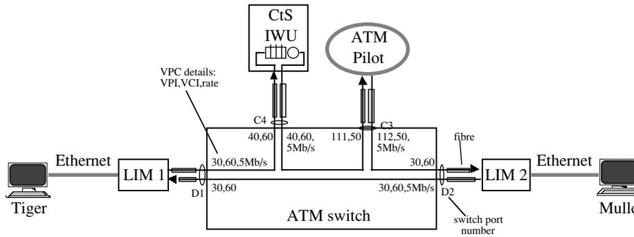
Figure 6 Configuration for varying shaper rates
