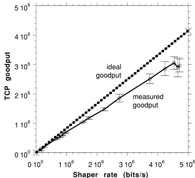
Graph 2 TCP goodput measured for varying shaper rates, with 95% confidence intervals.
