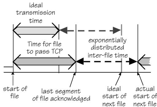
Figure A.2 Elongation of file transmission time due to TCP layer in the simulation model
