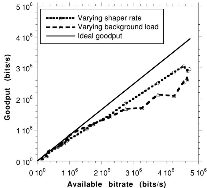
Graph 8 Comparison of throughputs by varying the shaper rate and the background rate
