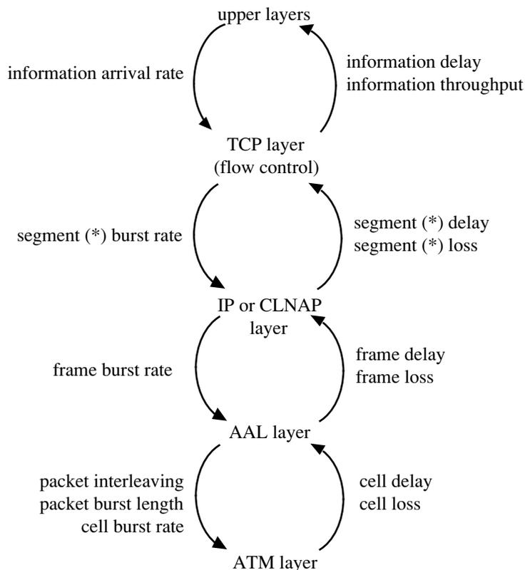
Figure 3 Interaction between different protocol layers
