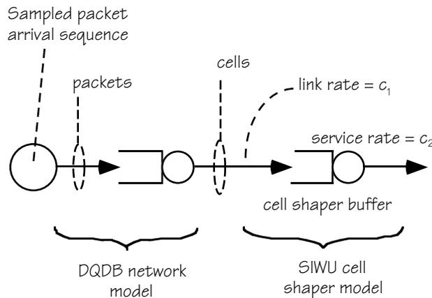
Figure B.1 Queueing model used for simulation of sampled traffic
