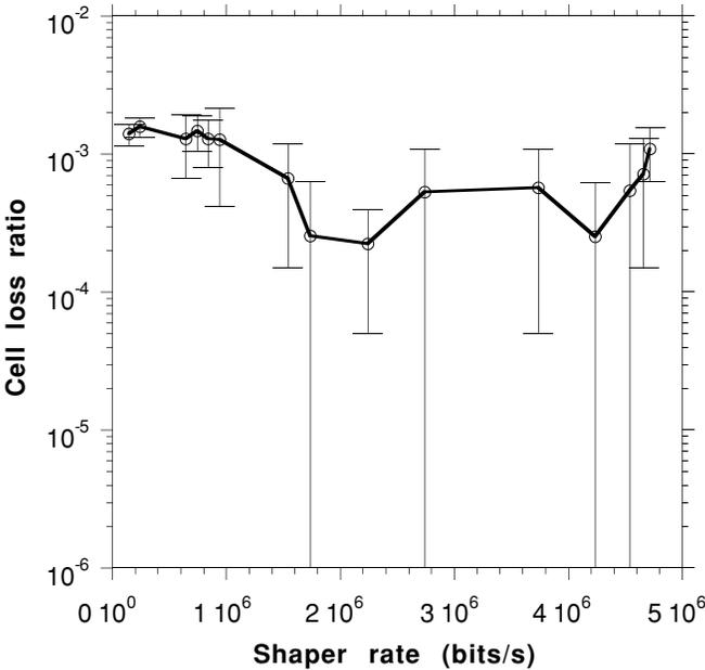
Graph 3 Cell loss ratio for different shaper sizes, with 95% confidence intervals
