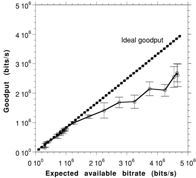
Graph 6 TCP goodput and ideal goodput for different available bitrates, taking into account the reduction of background bandwidth resulting from shaper cell loss.
