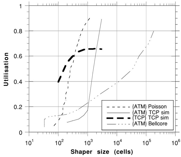
Graph 1 Comparison of dimensioning approaches for the shaping buffer
