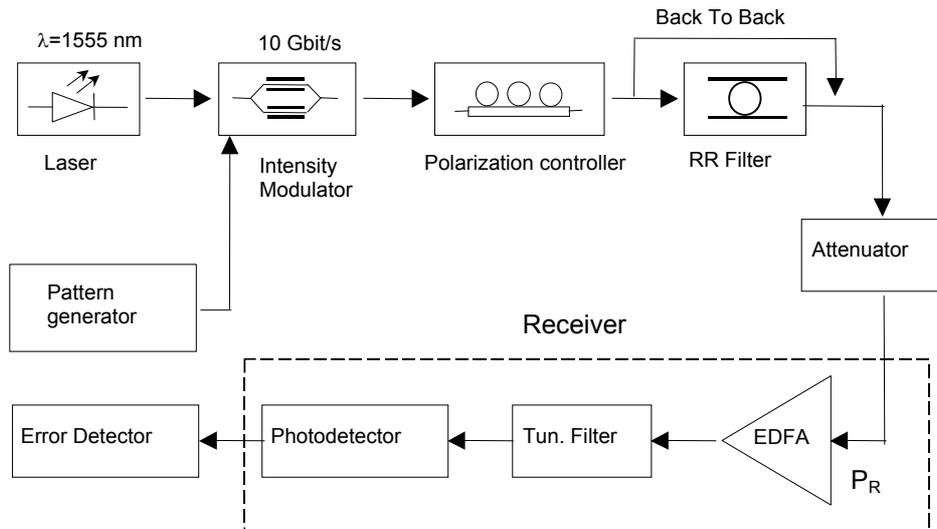
**Fig. 3.** Experimental set-up.  $P_R$  is the received power.
