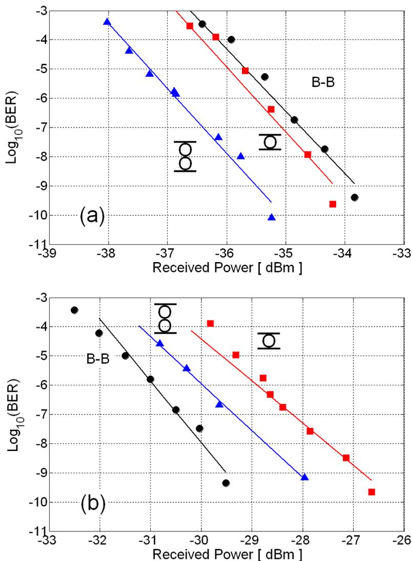
**Fig. 5.** *BER* of NRZ transmission at (a) 2.5 Gbit/s and (b) 10 Gbit/s (● Back to Back; ■ Single ring; ▲ Double ring).
