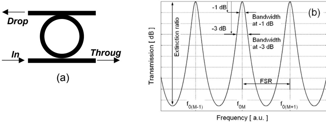
**Fig.1.** (a) Ports definition in a single resonator ring filter. (b) Typical single-ring drop port transfer function.
