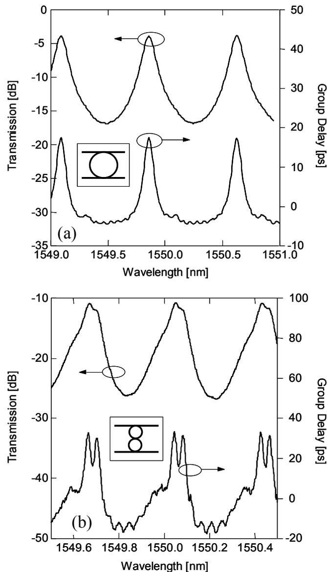
**Fig. 2.** Intensity and group delay characteristics of (a) the single and (b) the double ring-resonator.
