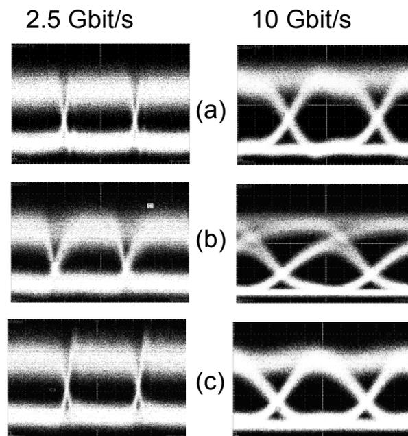
**Fig. 4.** 2.5 *Gbit/s* and 10 *Gbit/s* *NRZ* eye diagrams of (a) the *Back to Back*, (b) the single-ring filtered and (c) the double ring filtered sequence.
