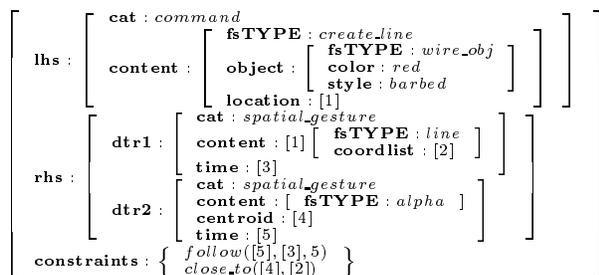
Figure 12: Rule Schema for Unimodal Barbed Wire
