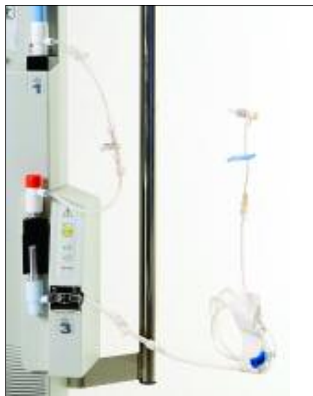
Figure 10. Level 1 H-1200 with integrated air detector/clamp (Smiths Medical, London, UK). The device consists of a heater that warms water and circulates it through a pump and a heat-exchange segment with a central tube (1) for water flow as in Figure 1 (countercurrent heat exchange technology). On detection of air in the line, the flow of blood and crystalloid is automatically stopped (3), allowing for removal of air and restoration of flow. There are audible and visual alarms when air is detected. The use of ultrasonic air detection coupled with automatic shutoff is a significant safety improvement.
