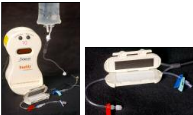
Figure 6, A and B. Belmont Buddy warmer (Belmont Instrument Corp., Bellerica, MA). The disposable set is attached close to the patient to minimize heat loss in the patient line. Priming volume is small (4 mL). The disposable set has microporous membranes that vent air from crystalloid fluid. Air is released through the side vents of the set to minimize the risk of air embolism.
