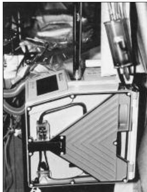
Figure 2. Belmont FMS 2000 warming system (Belmont Instrument Corp., Billerica, MA). The system consists of an integrated volumetric infusion pump coupled with a high-capacity magnetic induction heater. There are two ultrasonic air detectors, one at the fluid inlet and the other at the outflow to the patient coupled to an automatic shut off.
